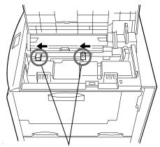
Toner Container Release Levers (Be sure to set to the left and fix the container in place.)
